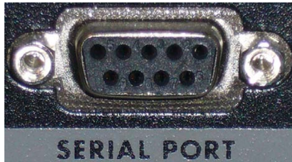
The female serial port, found on the back panel of an iScan VP xx video processor.
